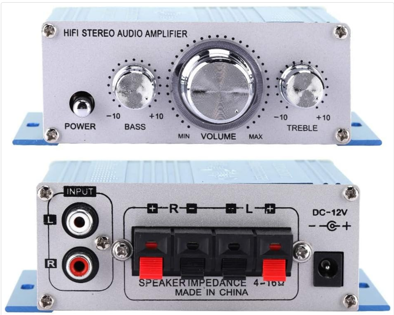
Figure 5.1: Front and rear view of the amplifier, illustrating the power input, audio input (RCA), and speaker output terminals. The front panel shows the Power button, Bass, Volume, and Treble control knobs.
