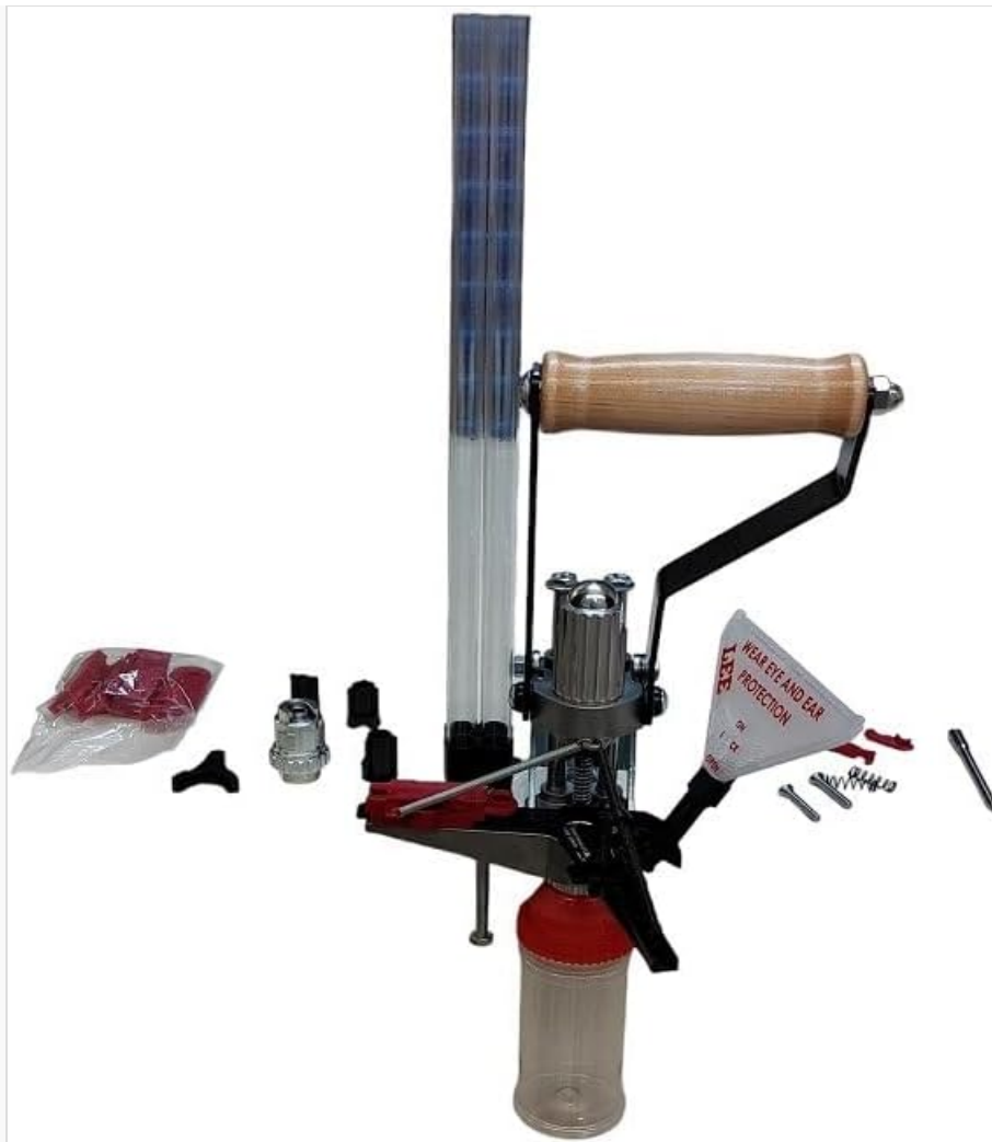
Image: Overview of the Lee Deluxe APP Press Kit, showing the press, roller handle, case feeder, and various accessories.
