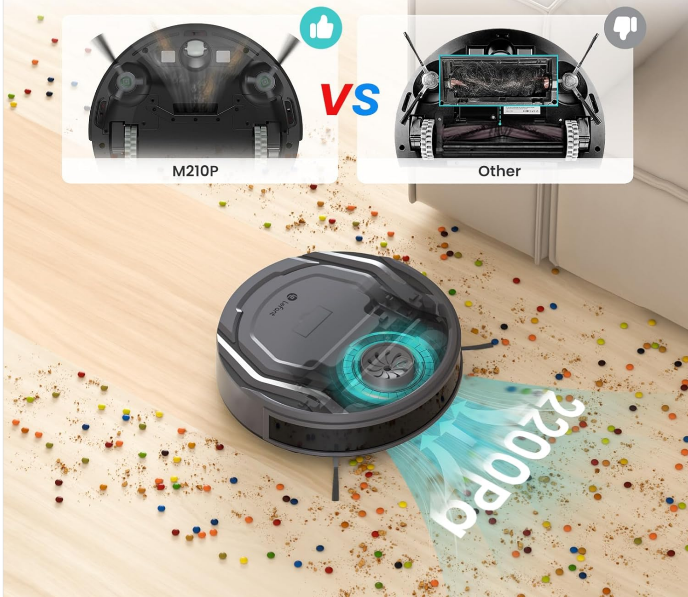
Figure 8: The brushless suction port design minimizes hair tangling compared to traditional roller brushes.
