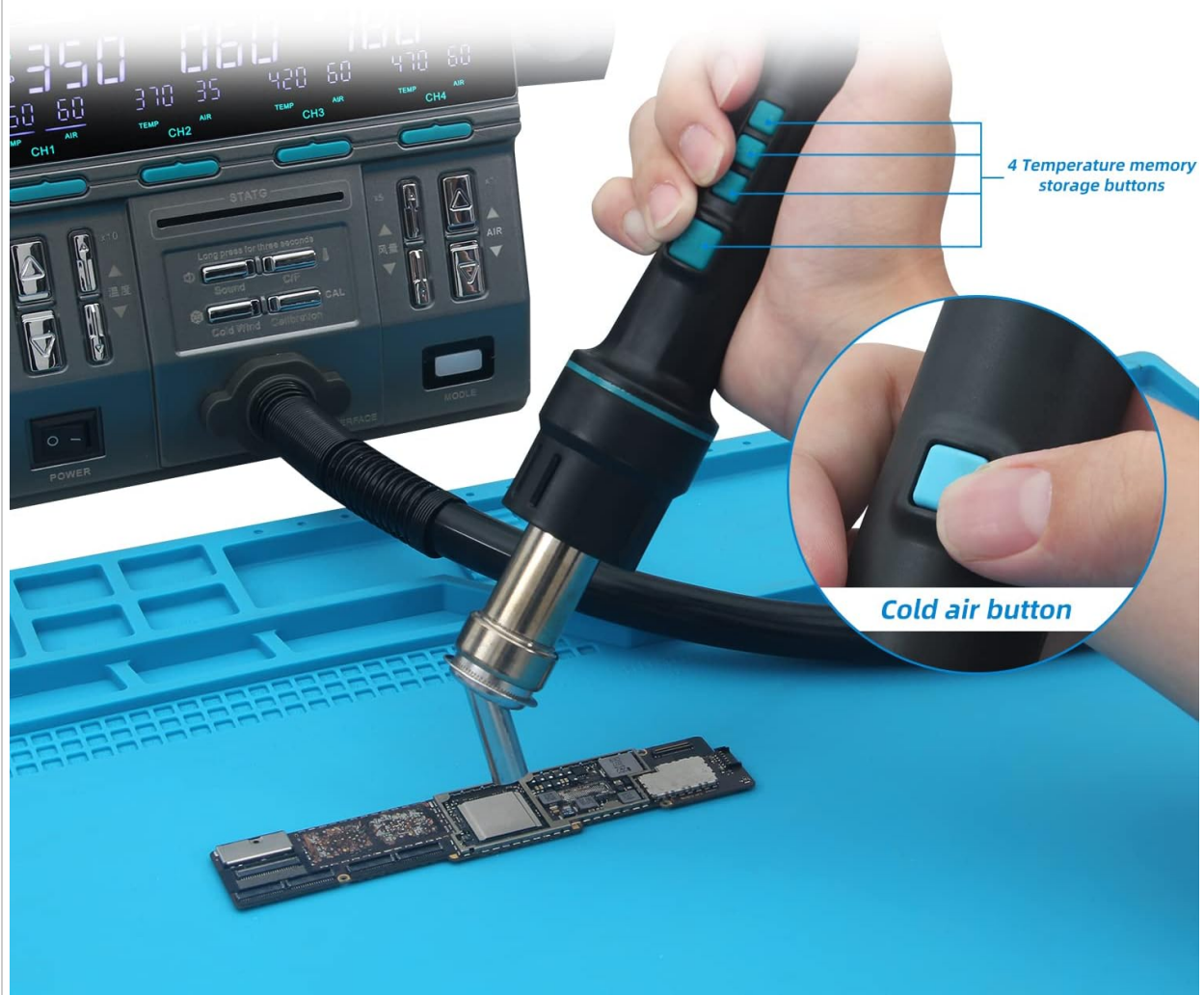
Figure 6: Hot air gun handle with memory and cold air buttons.
