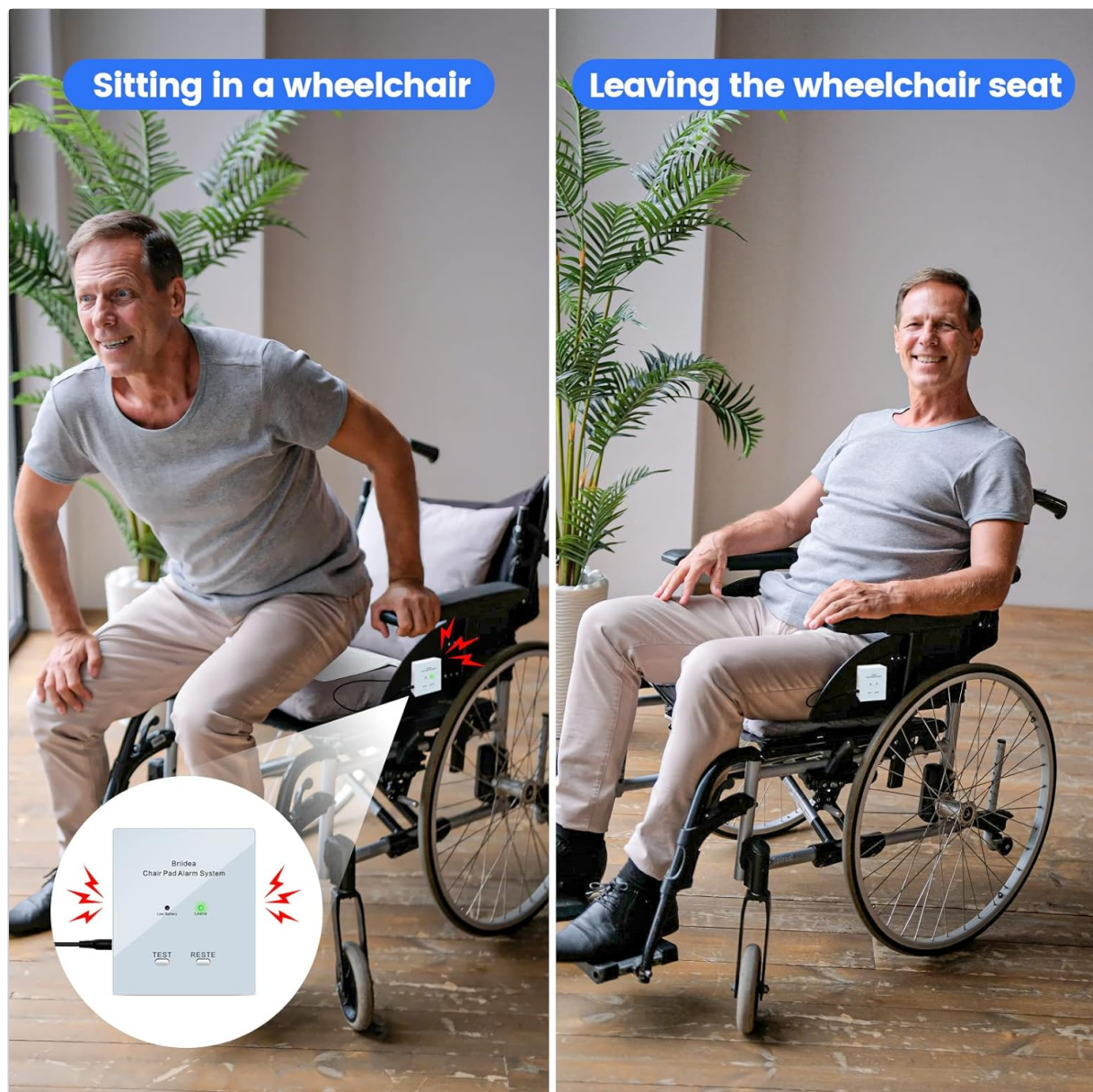
Figure 4.1: Illustration of the alarm activation when a user leaves their wheelchair seat.
