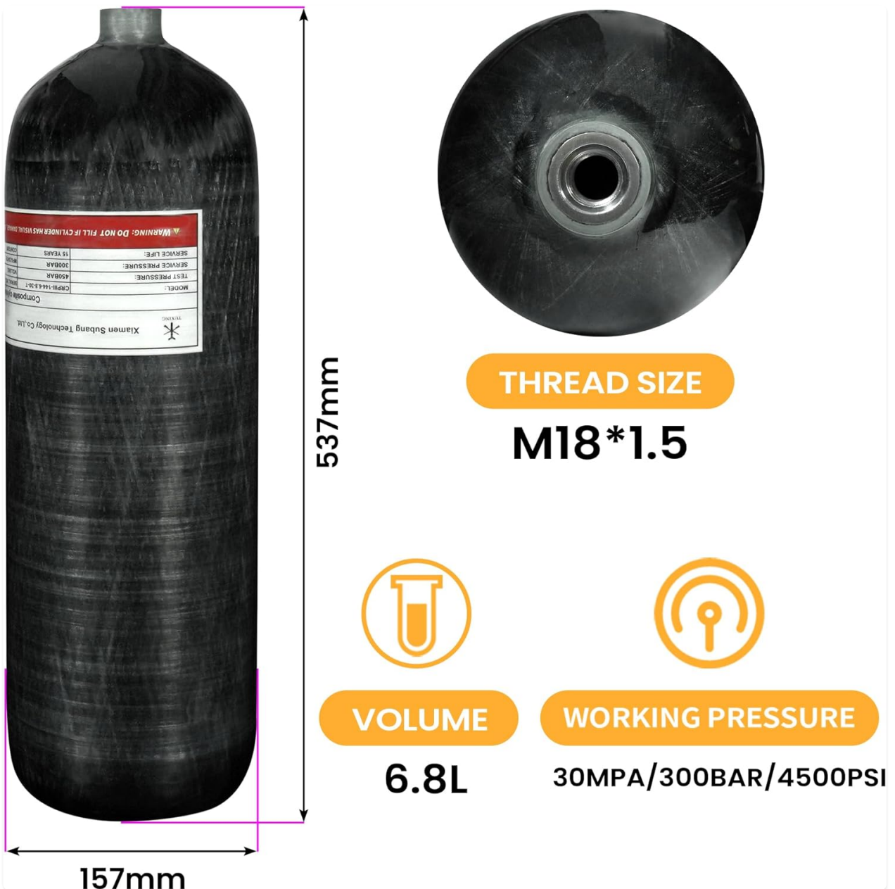
Figure 7: Tank Dimensions and Thread Size
