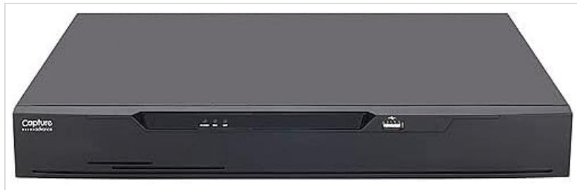
The image displays the front panel of the Capture Advance R2-HDDVR8C2T DVR. It is a black, rectangular unit with a sleek design. On the left side of the front panel, the "Capture Advance" logo is visible. Towards the center, there are three small indicator lights, likely for power, HDD activity, and network status. On the right side, a USB port is present for connecting a mouse or USB drive. The overall appearance is compact and suitable for desk, rack, or wall mounting.
