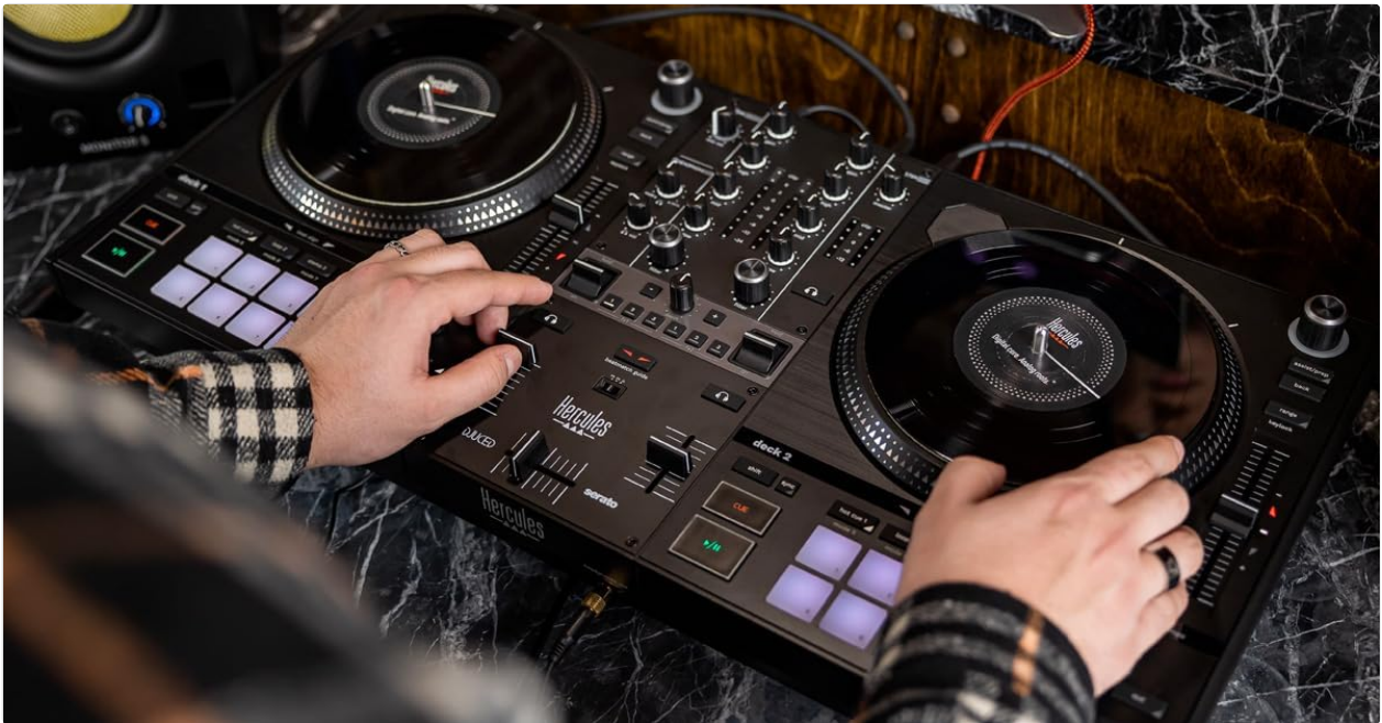
Figure 3: Hands-on operation of the DJControl Inpulse T7, demonstrating interaction with the motorized platters and mixer section.
