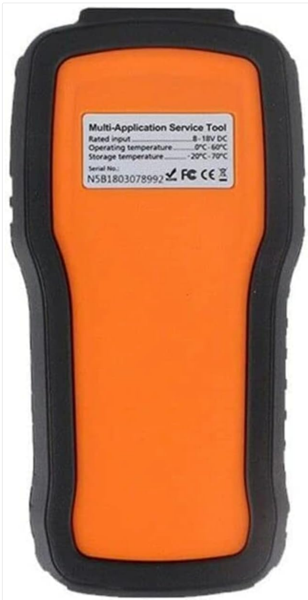
Figure 7.1: Device Specifications. The label on the back of the device provides details such as rated input, operating
