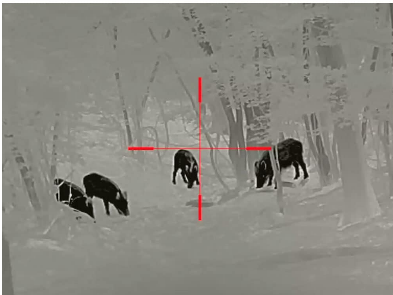
Figure 5.1: Thermal image display in 'White Hot' palette, showing target animals with a red aiming reticle.
