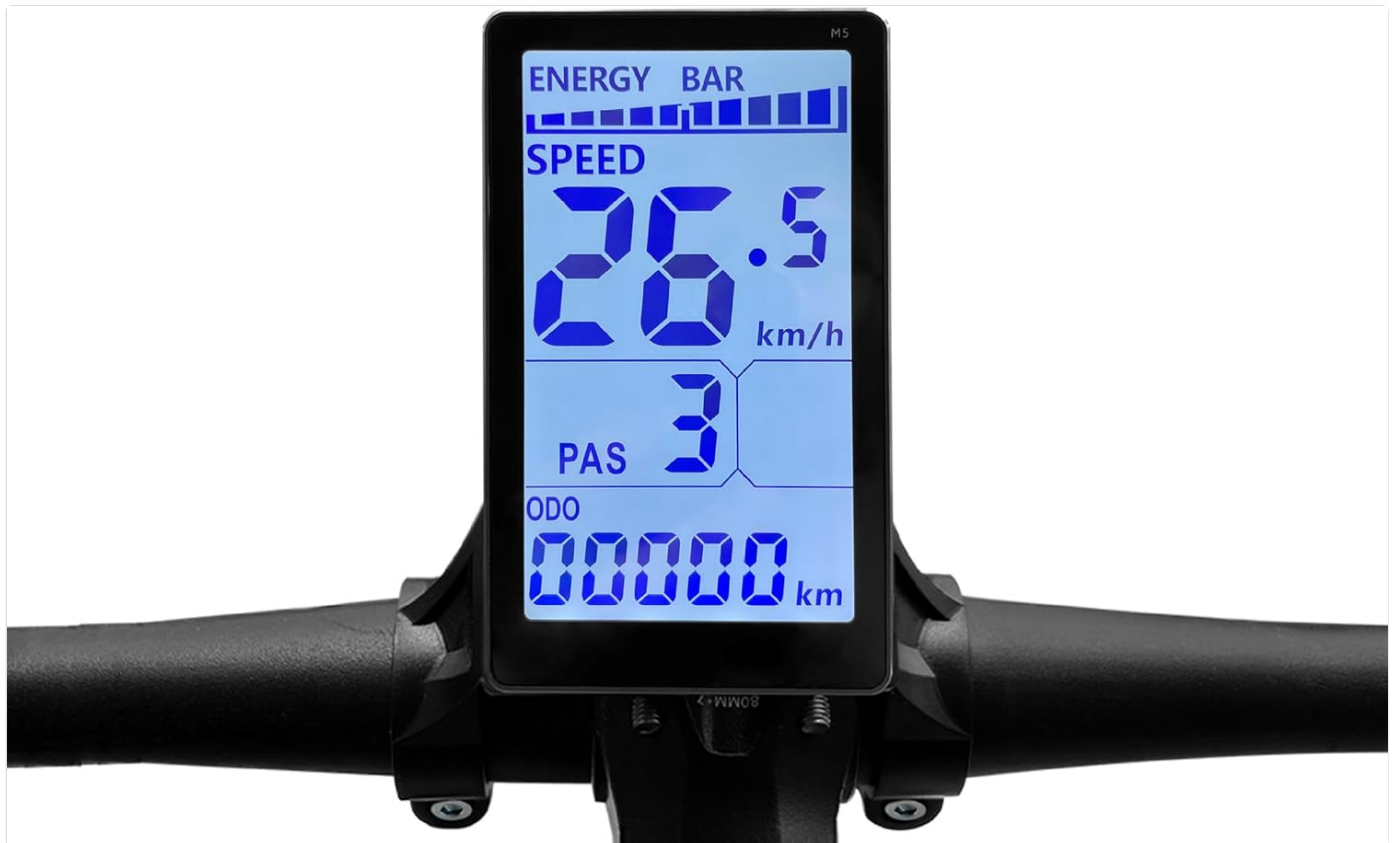
Image: The M5 LCD Display showing various data points including speed, pedal assist level, and odometer reading.
