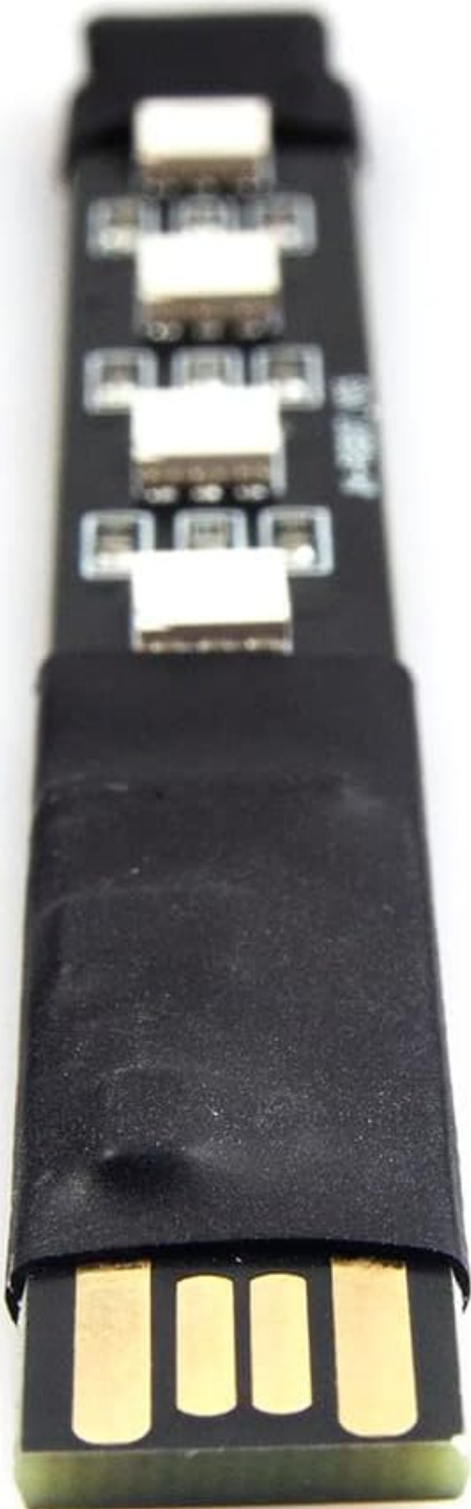
Image: Close-up view of the USB-A male connector end of the REXUS USB LED controller.
