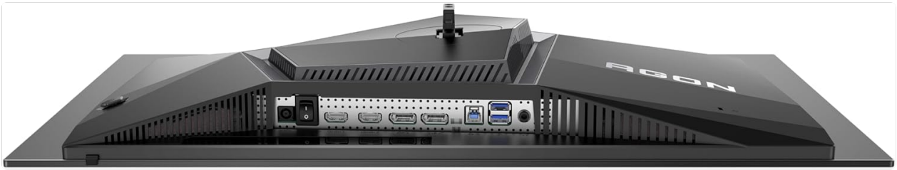
Figure 4.3: Monitor input/output ports.
