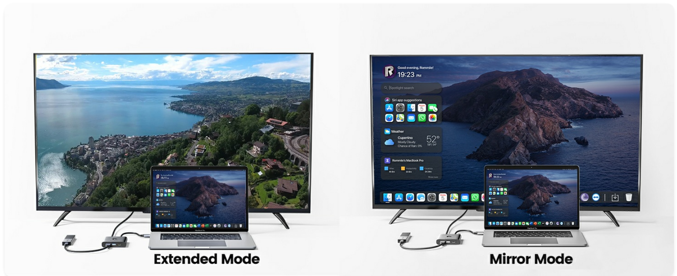
Figure 6: Extended Mode and Mirror Mode display options.
