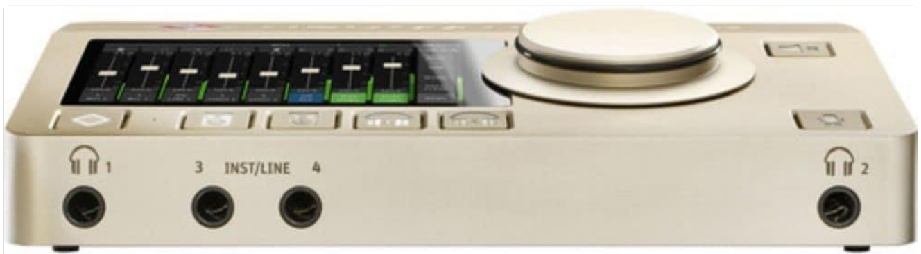
Image: The front of the Neumann MT 48, featuring two headphone jacks and two instrument/line inputs for easy access during recording sessions.
