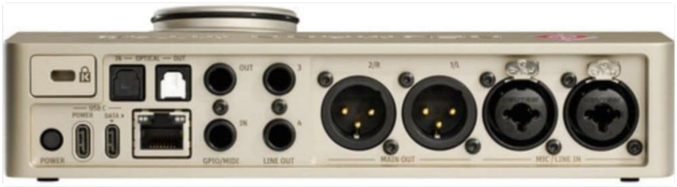
Image: The rear panel of the Neumann MT 48, highlighting the diverse range of connectivity options including XLR/TRS combo inputs, line outputs, optical I/O, MIDI, and USB-C ports.
