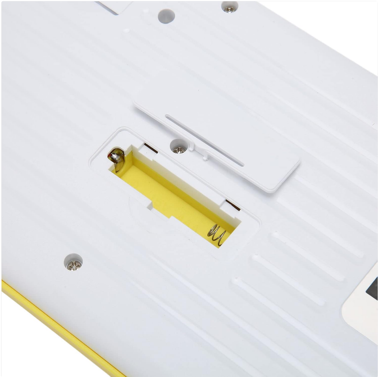
Image: The underside of the EBTOOLS keyboard with the battery compartment open, showing where to insert the AA battery.
