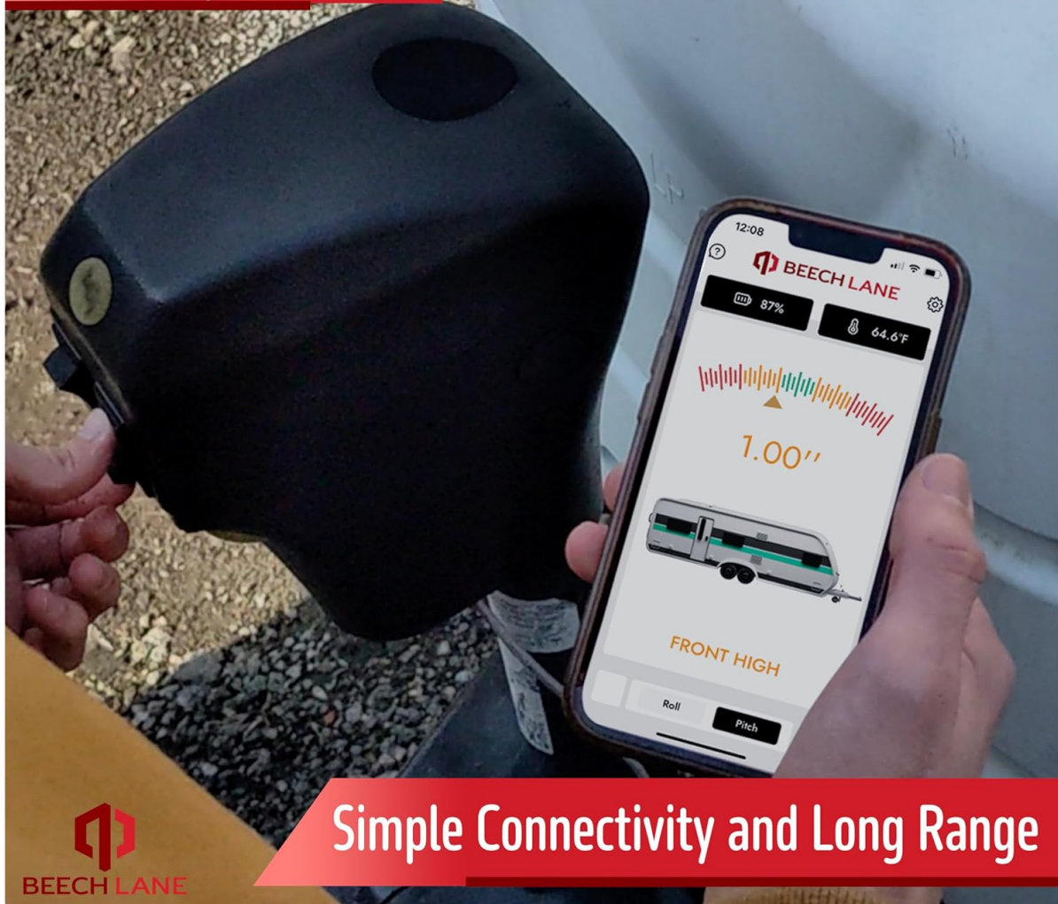
Figure 6: Adjusting RV level while monitoring the app.
