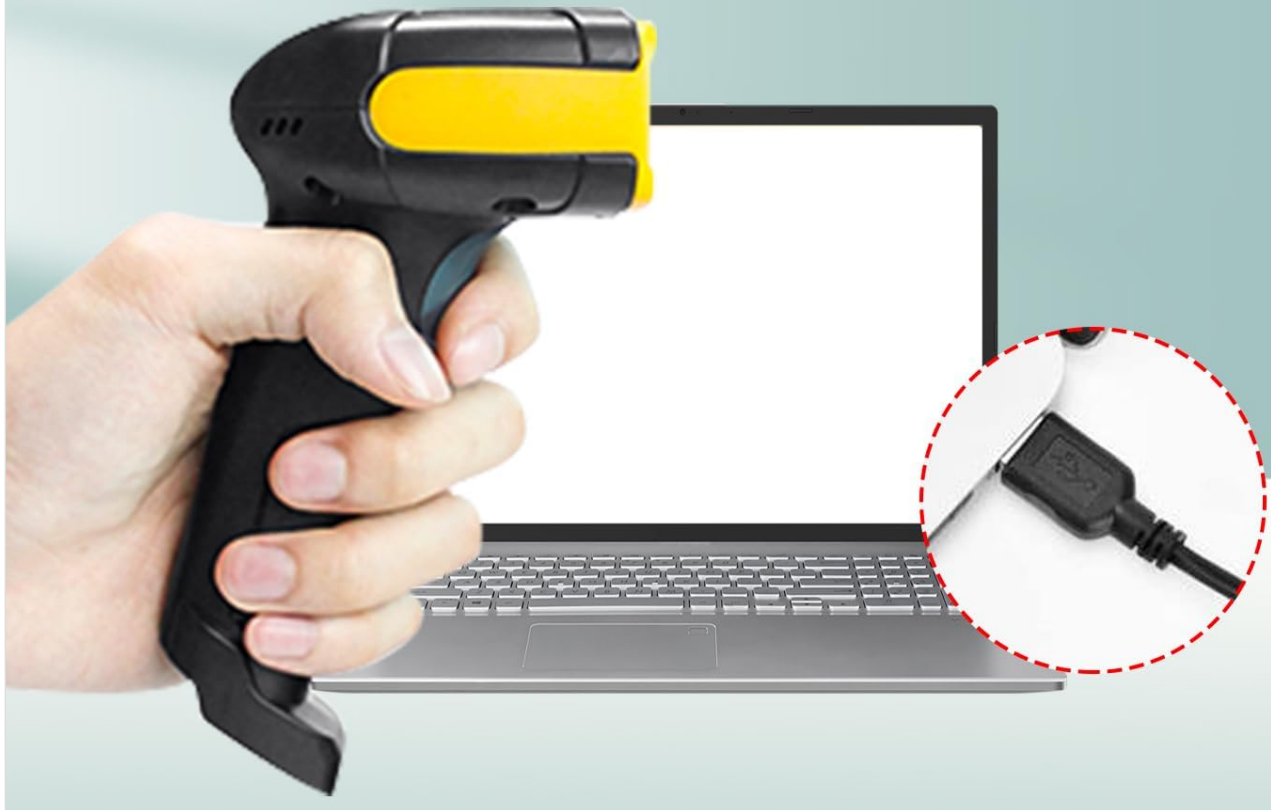
Figure 2: Plug & Play setup. The scanner connects directly to a PC or laptop via USB without needing driver installation. Note: Not compatible with iPhone or iPad.
