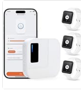
Figure 4: The emergency alert process involves pressing the SOS button, which triggers an audible alarm on the receiver and sends a notification to linked mobile phones.
