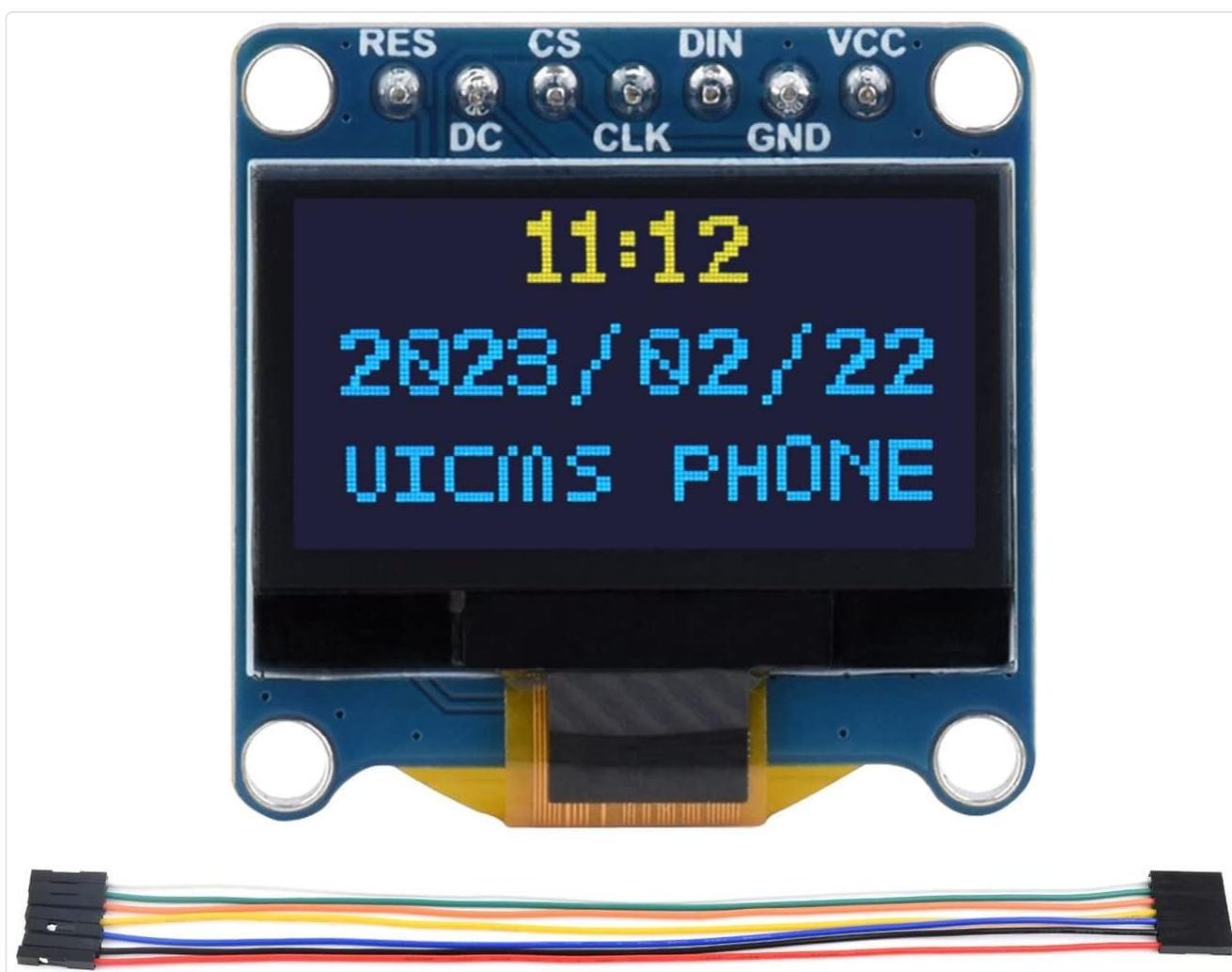
Image: The 0.96inch OLED Module shown with the included 7-pin female-female jumper cable.
