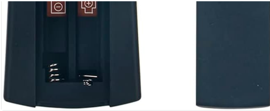
Figure 2: Battery compartment of the remote control. This image illustrates the open battery compartment on the back of the remote, clearly showing the two slots for AAA batteries and the polarity indicators.
