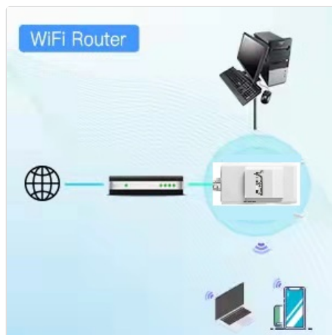
Image: Diagram showing the VAP11AC configured as a WiFi Router, providing internet access to various devices.
