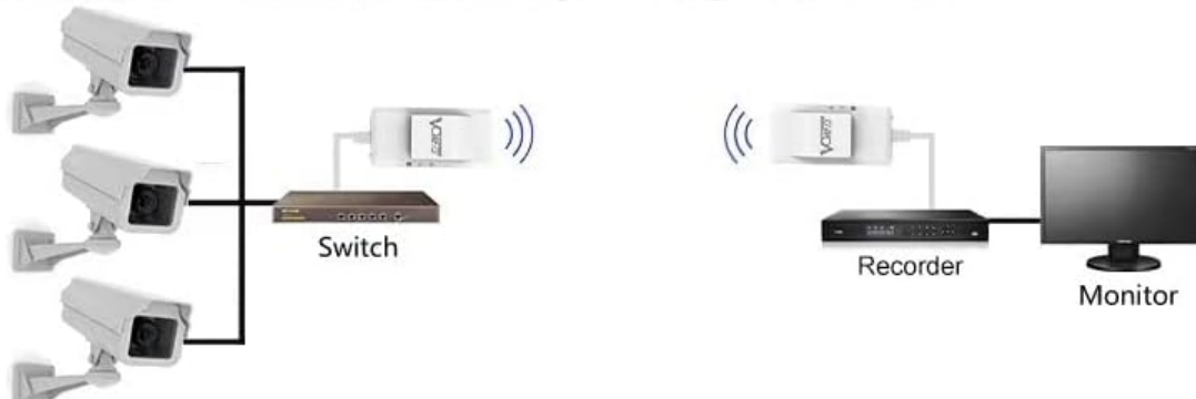
Image: Diagram illustrating various wireless monitoring application solutions, including point-to-point and multipoint wireless connectivity for surveillance cameras and DVRs.
