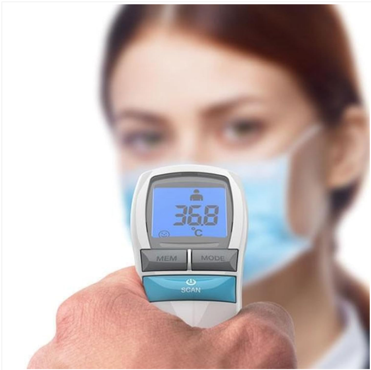
Figure 3: Demonstrates the Homedics TE-200-EEU being used to measure a person's forehead temperature, showing the non-contact method.
