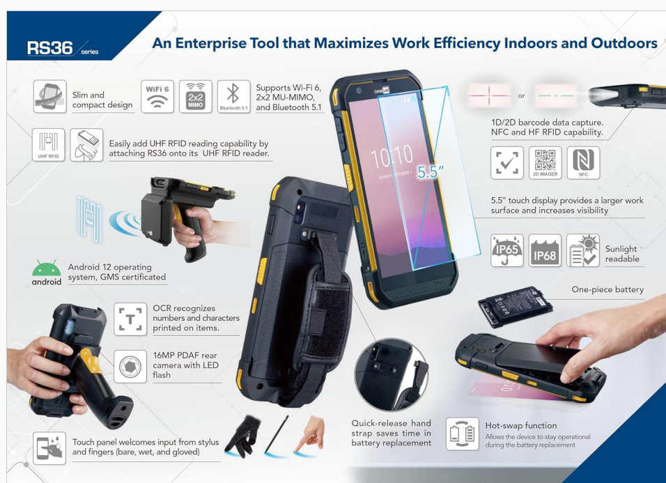
Figure 3.1: Battery Access. This image illustrates the battery compartment and the hot-swap feature, allowing for battery replacement without interrupting device operation.
