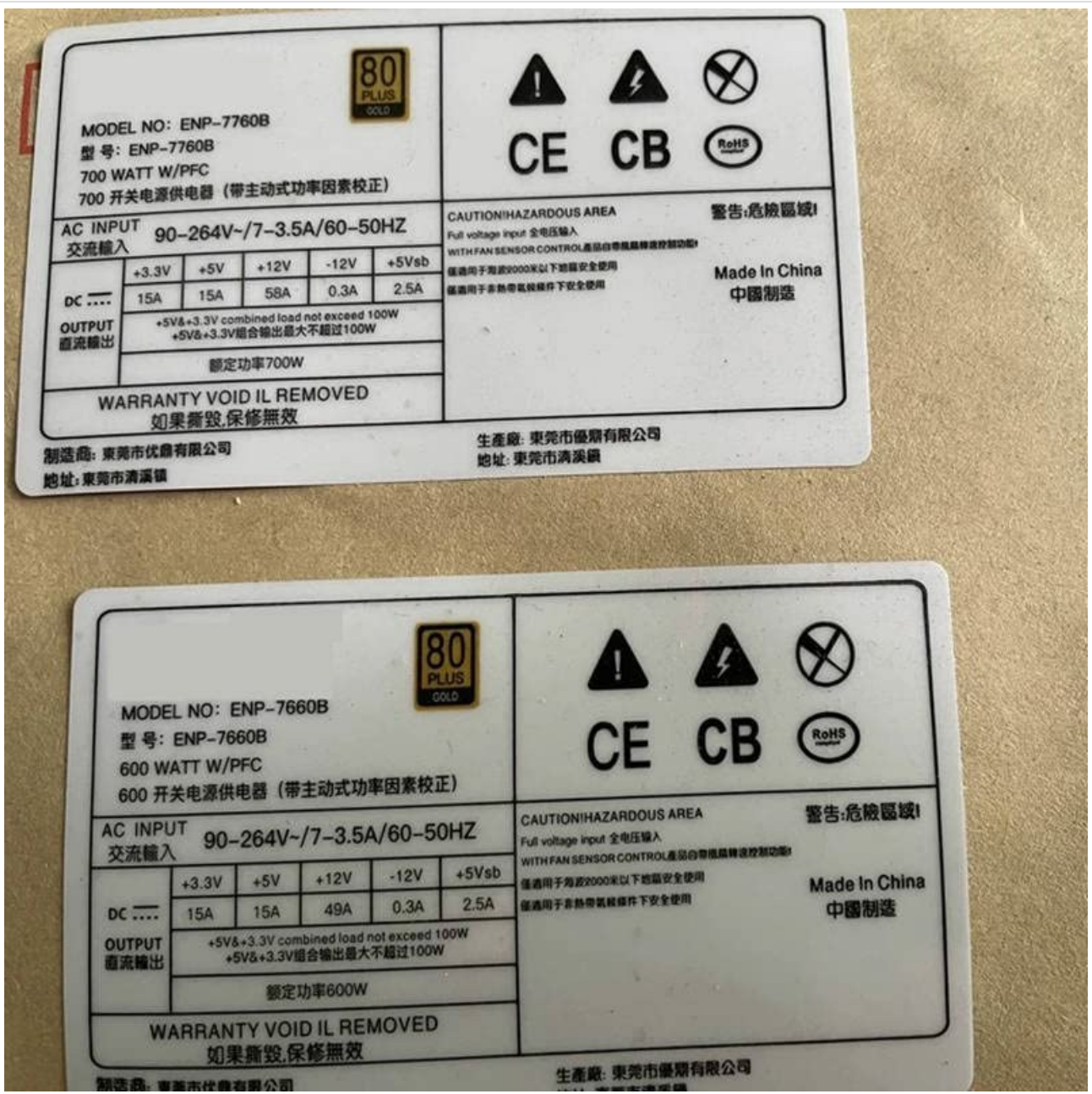
Figure 7.1: Specification label for the MIDTY ENP-7660B Power Supply Unit, detailing electrical input and output ratings, and certifications.
