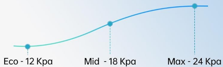
Figure 2.2: Brushless Motor and Suction Power Modes.
