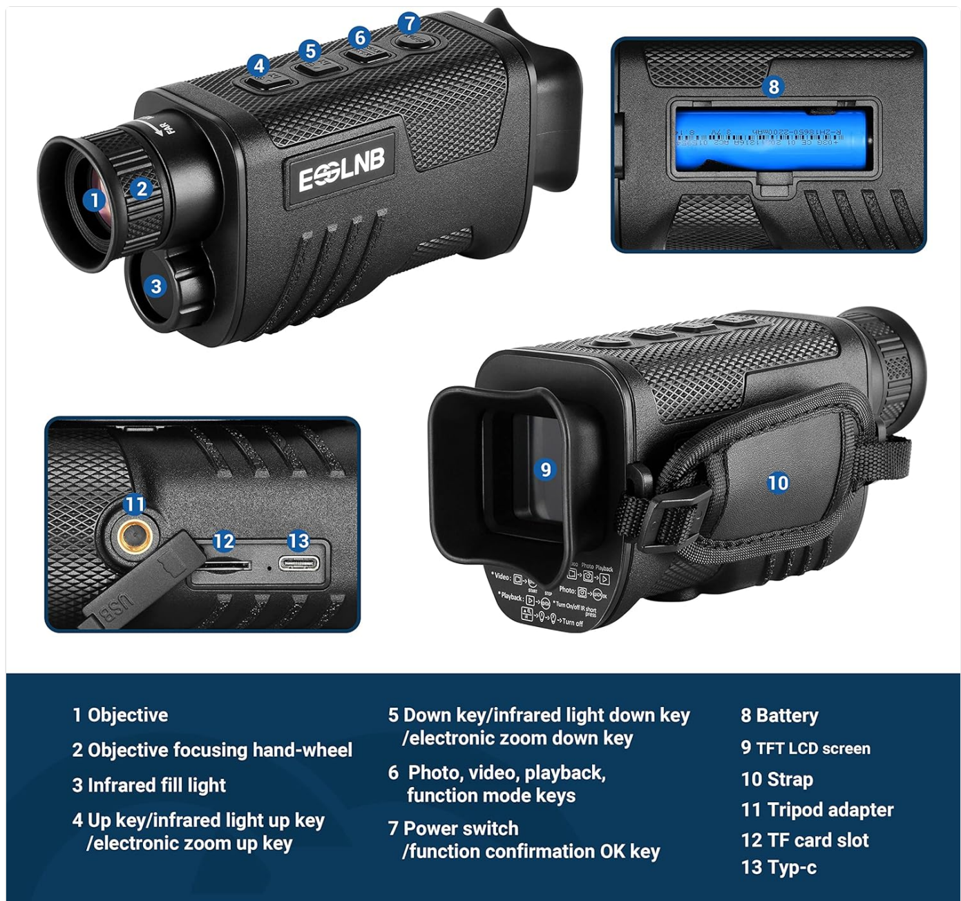
Figure 2.1: Monocular Components Diagram
