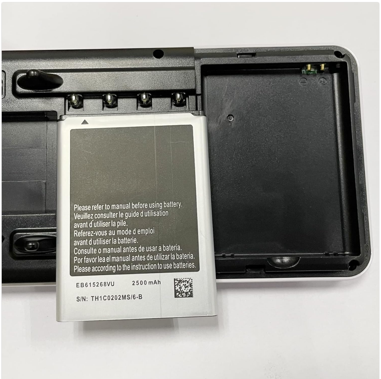
Image 3.1: Close-up view of the battery being inserted into the magnifier's battery compartment.
