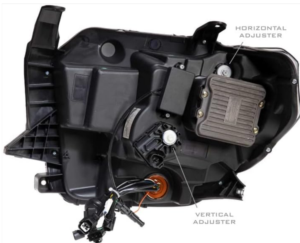
Image 5.1: Rear view of the headlight assembly, indicating the locations of the horizontal and vertical adjustment screws.
