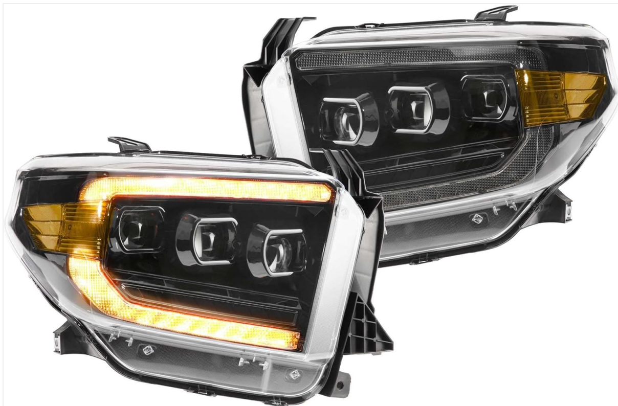
Image 1.1: Pair of Morimoto XB LED Headlight Assemblies, showcasing the amber DRL strip and projector lenses.
