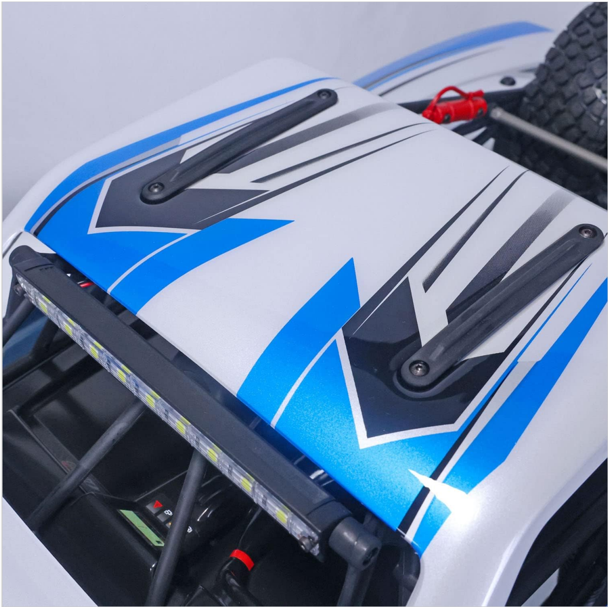
Figure 6.1: Top view of the DF7 V2, highlighting the roof-mounted light bar.
