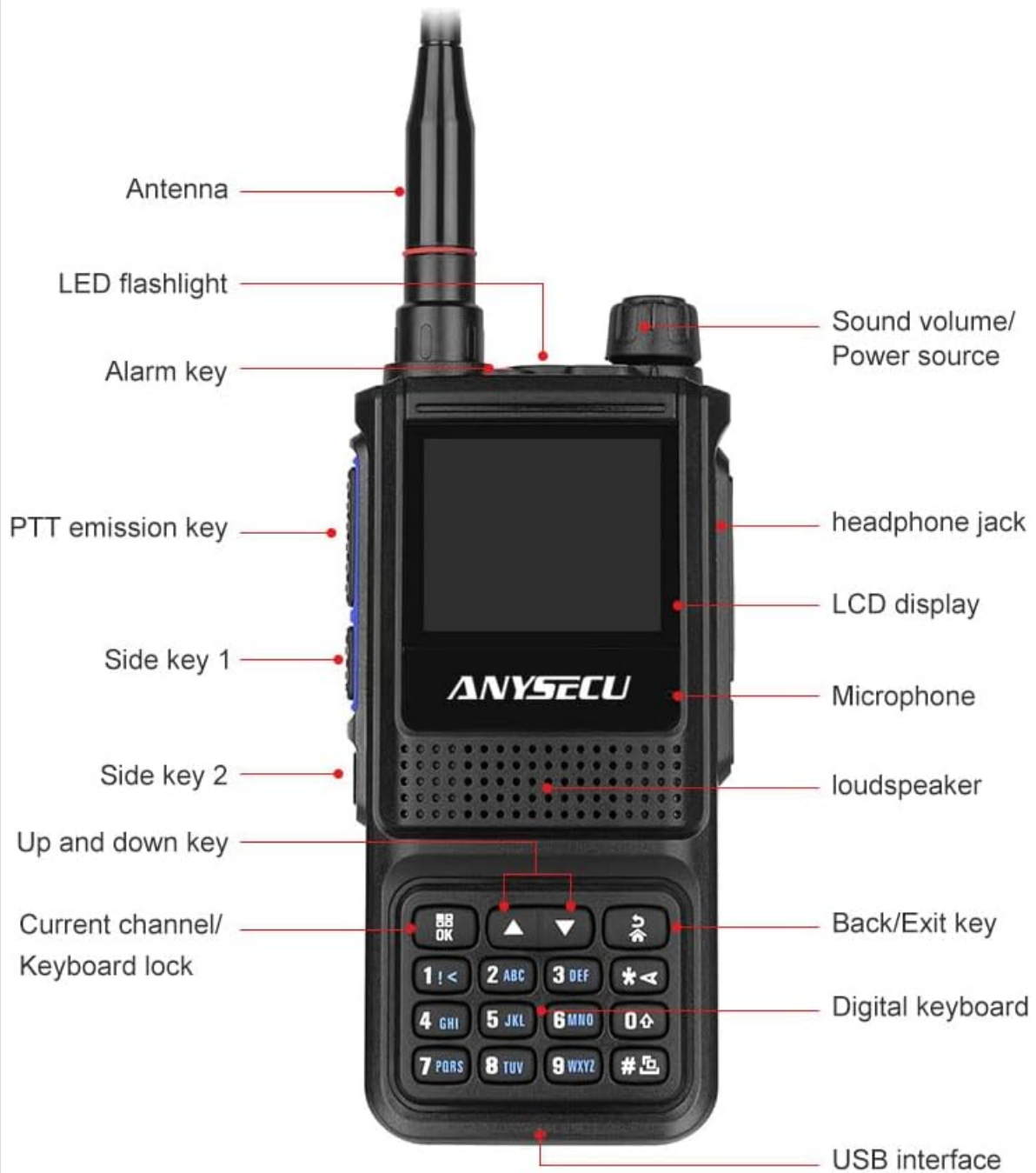
Image: Detailed diagram labeling the various parts of the Anysecu AC-881 walkie talkie, including Antenna, LED flashlight, Alarm key, PTT emission key, Side key 1, Side key 2, Up and down key, Current channel/Keyboard lock, Digital keyboard, Back/Exit key, USB interface, Sound volume/Power source, Headphone jack, LCD display, Microphone, and Loudspeaker.
