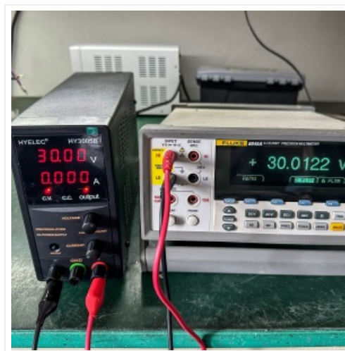
Figure 2.2: Detailed view of the 4-digit LED display on the HYELEC HY3005B, showing voltage and current readings with high precision and stability.
