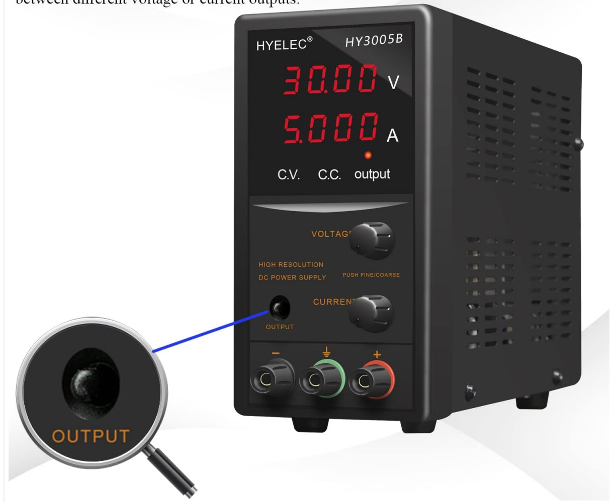
Figure 4.1: Close-up of the output switch on the HYELEC HY3005B, designed to prevent damage by allowing voltage and current settings before connecting the load.
