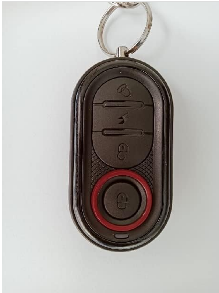
Figure 4.1: Close-up of the STEELMATE 986E remote control, showing its buttons for various functions.
