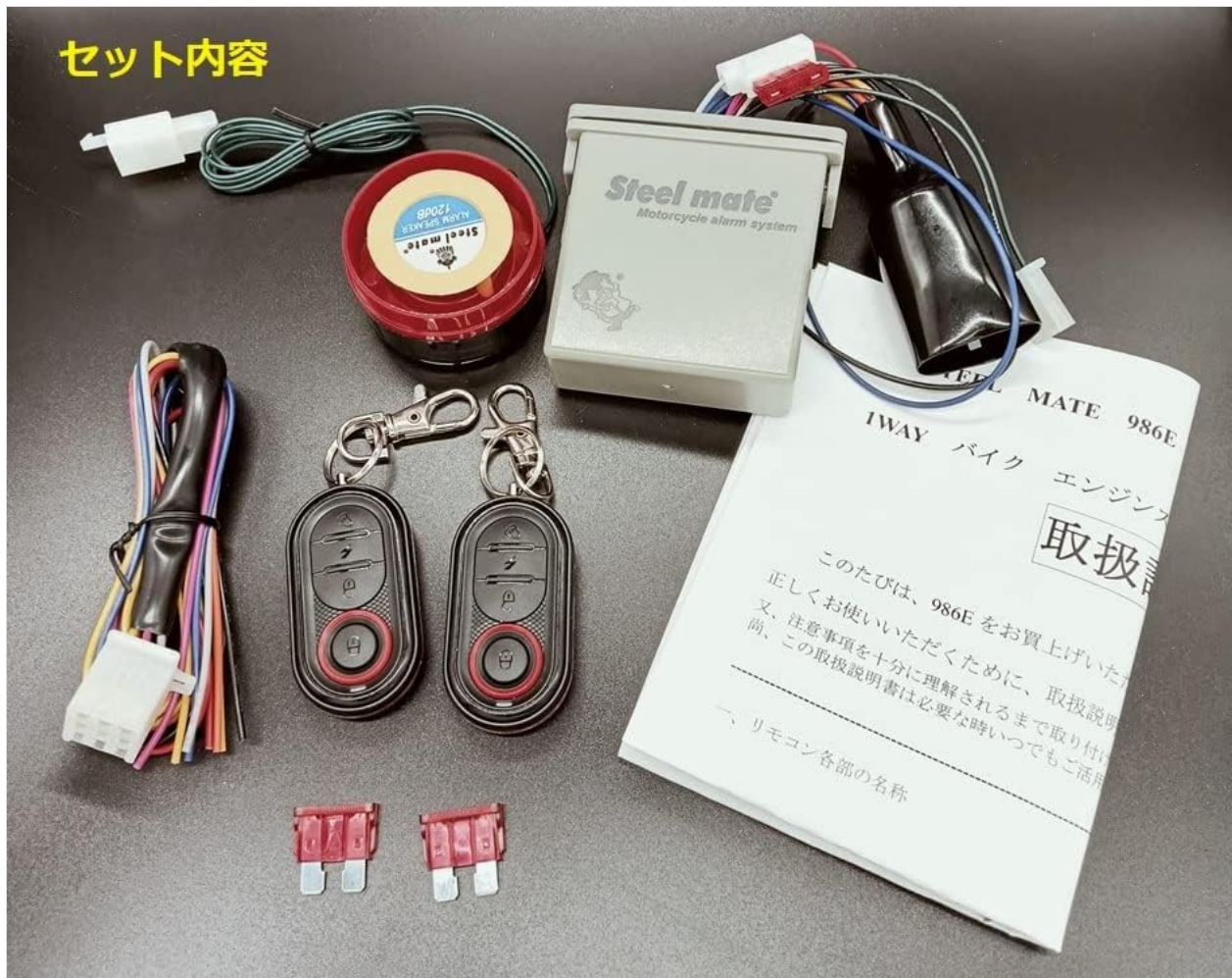
Figure 3.1: All included components of the STEELMATE 986E system, including the main unit, siren, remote controls, wiring, fuses, and the instruction manual.
