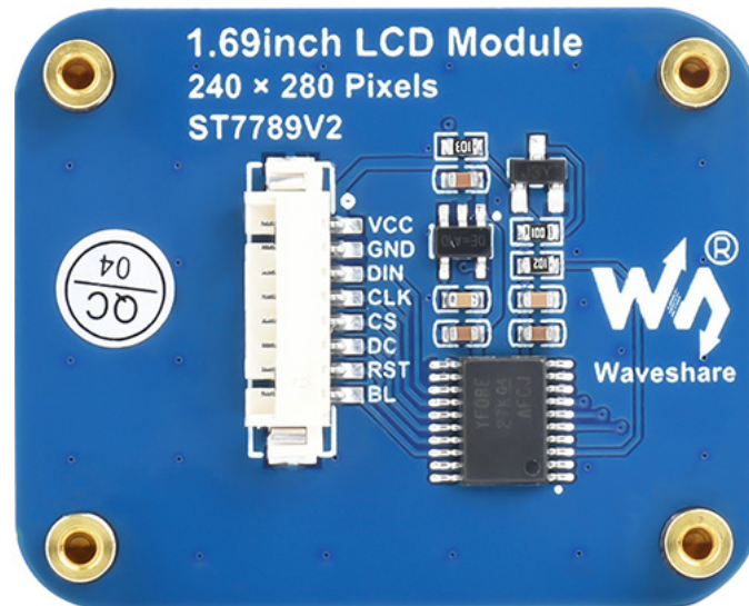
Image: The SPI control interface and pin definitions on the module.
