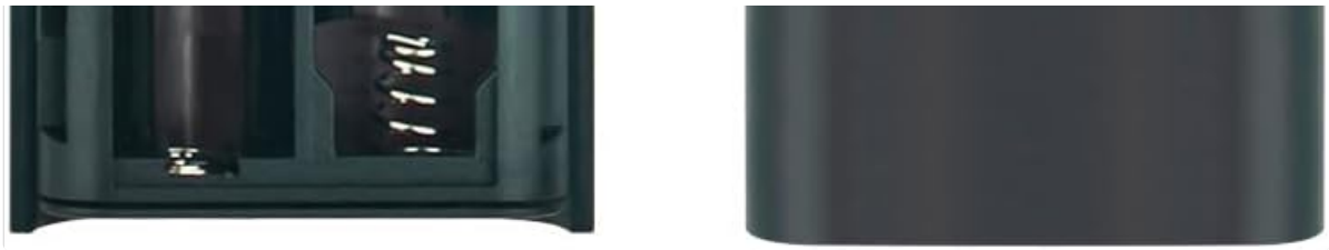
Figure 3.1: View of the battery compartment with two AAA batteries inserted, and the battery cover removed.
