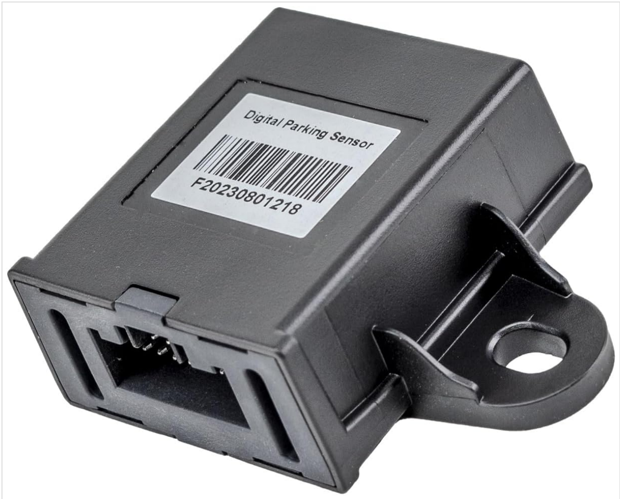
Image 2: The Electronic Control Unit (ECU) with a barcode label F20230801218. This unit processes sensor data and controls the display and speaker.
