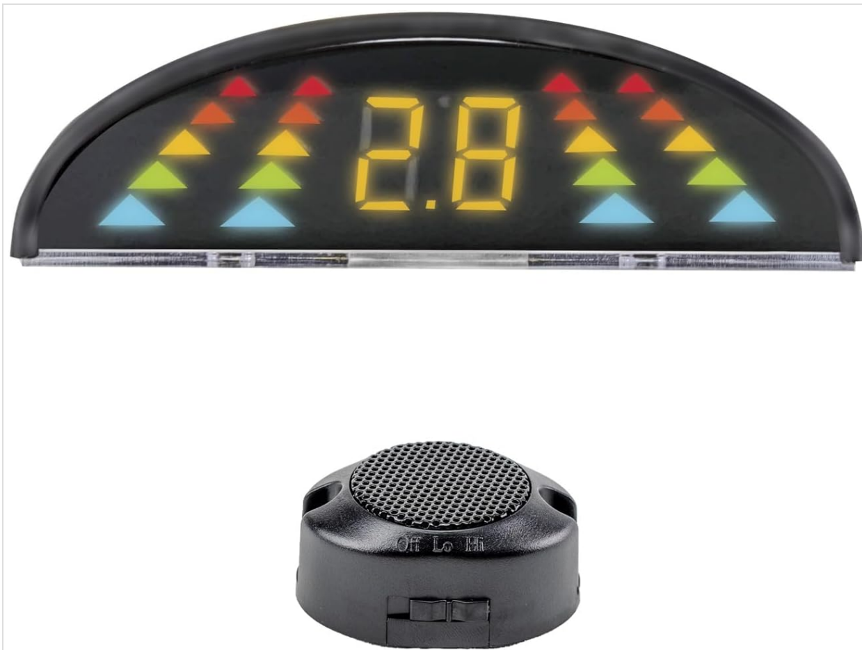
Image 3: The LED display unit. It shows numerical distance to an object and uses color-coded segments (green, yellow, red) to indicate proximity.
