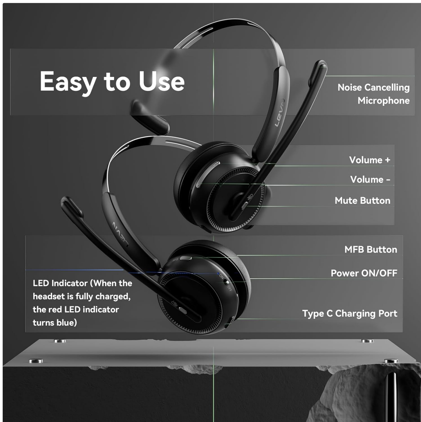
Figure 2: Detailed view of headset controls and ports. The LED indicator turns blue when fully charged.
