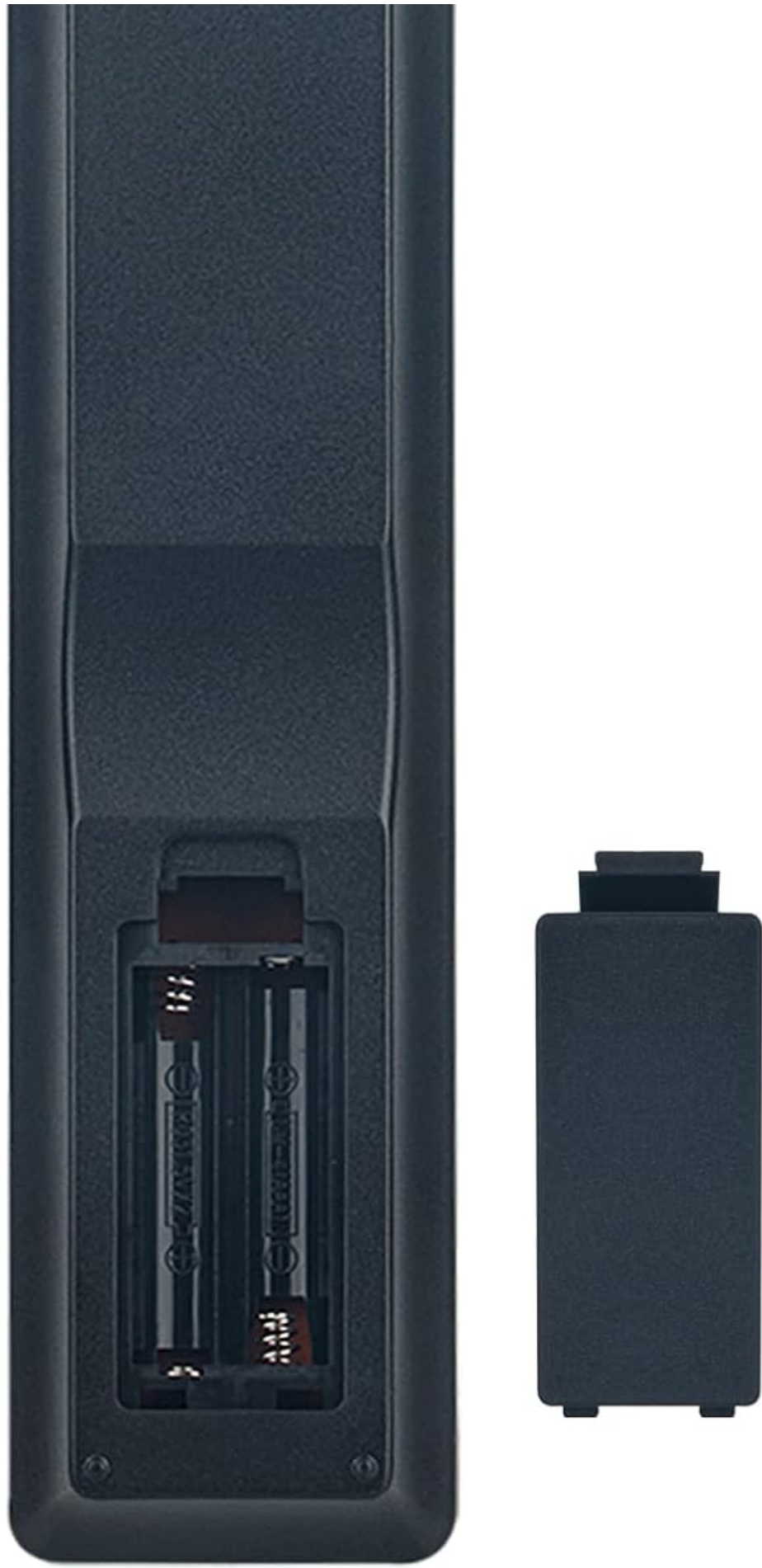
Figure 2: Rear view of the RC042SR remote control, illustrating the battery compartment with the cover removed.
