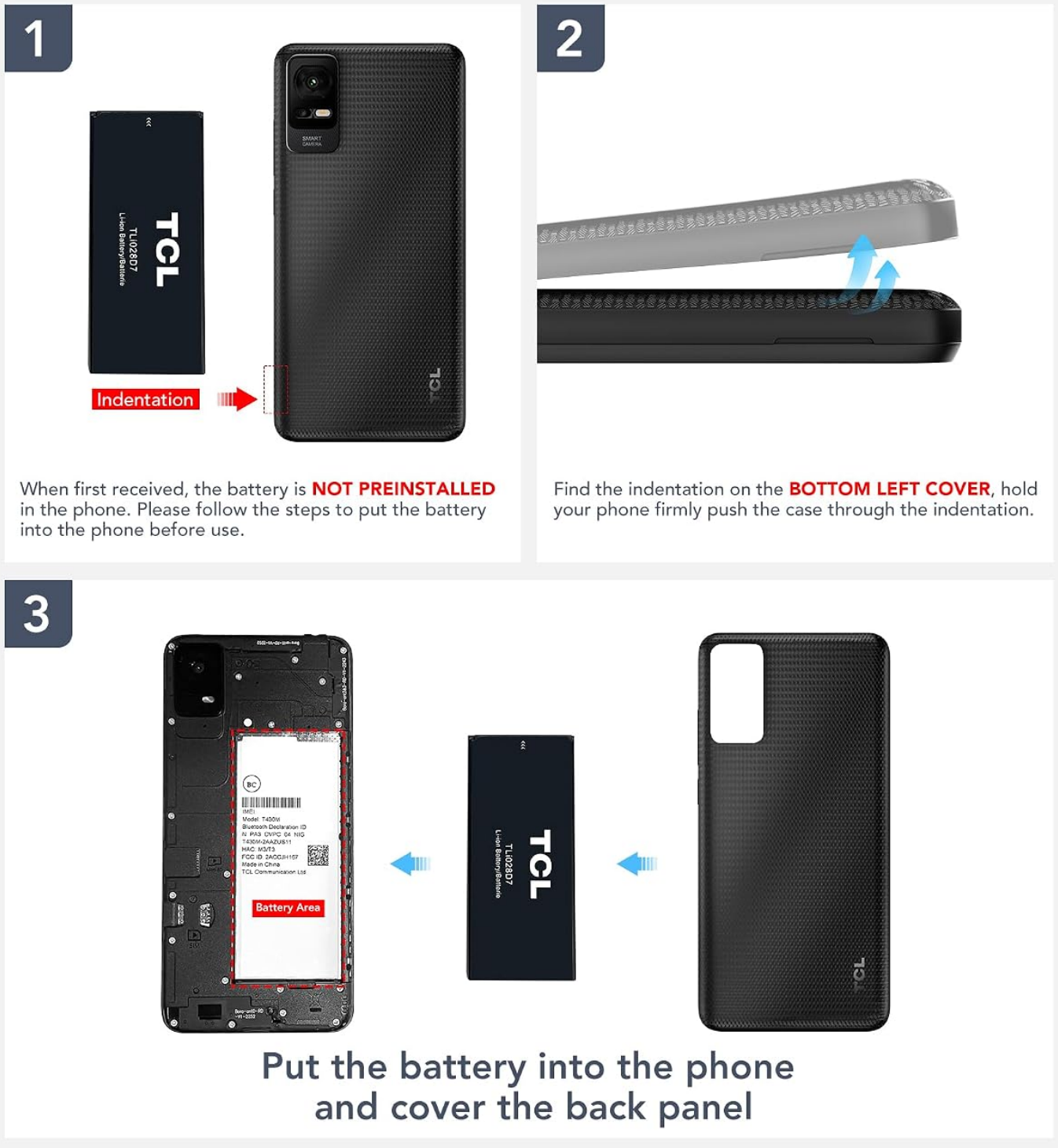
Figure 5.1: Visual guide for installing the battery. Step 1 shows the battery and phone back. Step 2 illustrates opening the back cover. Step 3 shows placing the battery and reattaching the cover.
