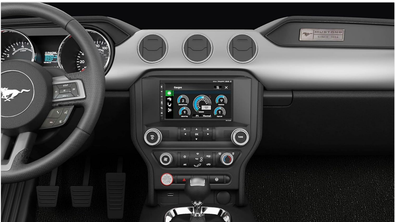
Image 6.2: An installed Pioneer modular receiver displaying various performance gauges within the Ford Mustang dashboard.
