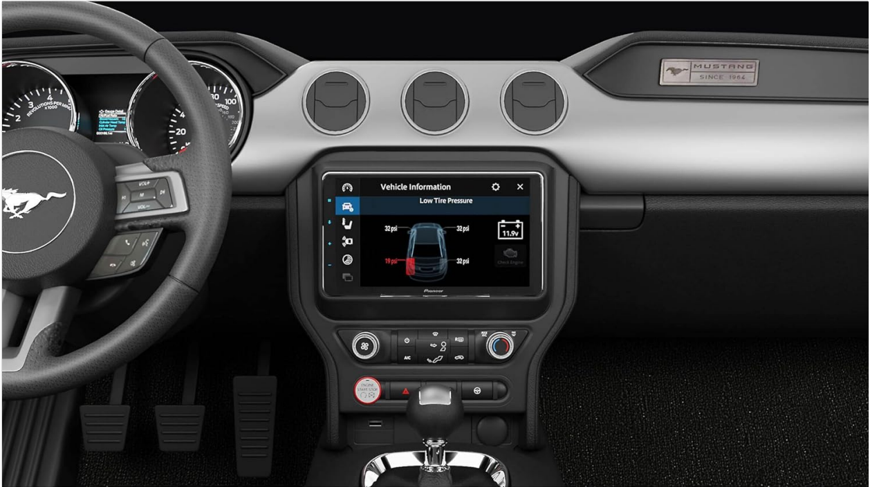
Image 6.1: An installed Pioneer modular receiver displaying vehicle information, including tire pressure, within the Ford Mustang dashboard.
