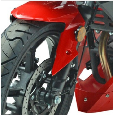
Image 4.2: Front wheel with disc brake assembly.
