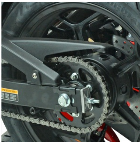
Image 4.3: Rear wheel with chain drive and disc brake assembly.
