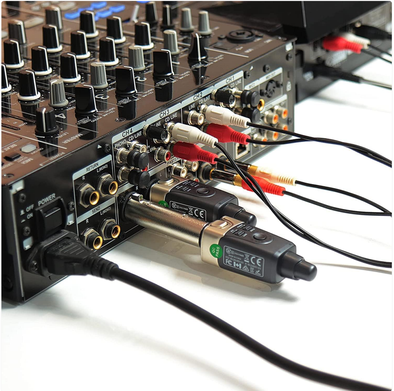
Figure 4.2: Receivers connected to a mixer for stereo output.
