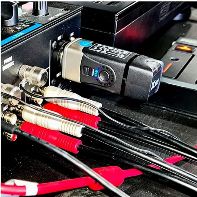
Figure 4.1: Transmitter connected to a microphone, receiver connected to a mixer.
