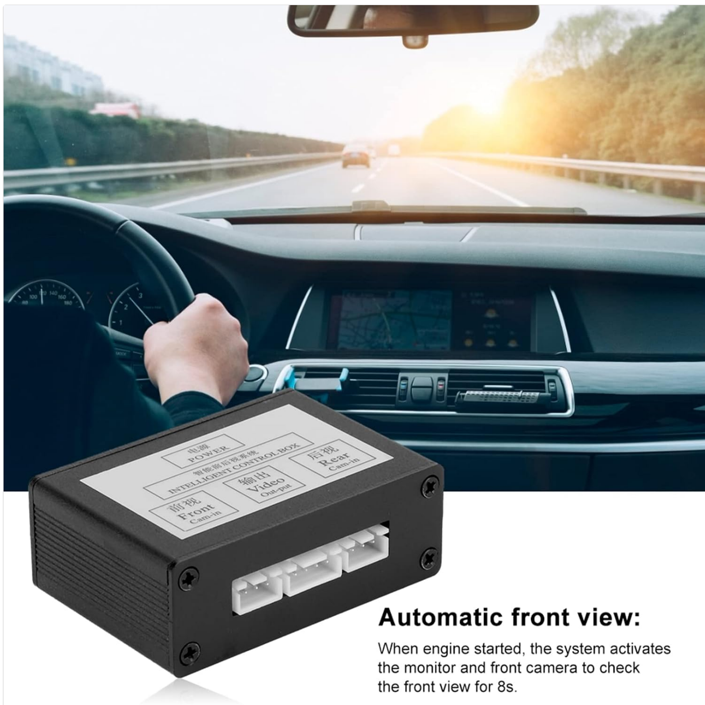
Image 6.1: Depiction of the automatic front view activation feature when the engine is started.
