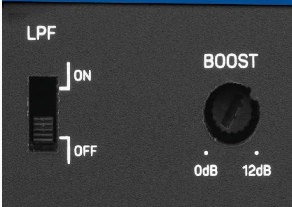
Image 5.3: Close-up of the Bass Boost knob (0dB to 12dB) and the LPF (Low Pass Filter) ON/OFF switch.
