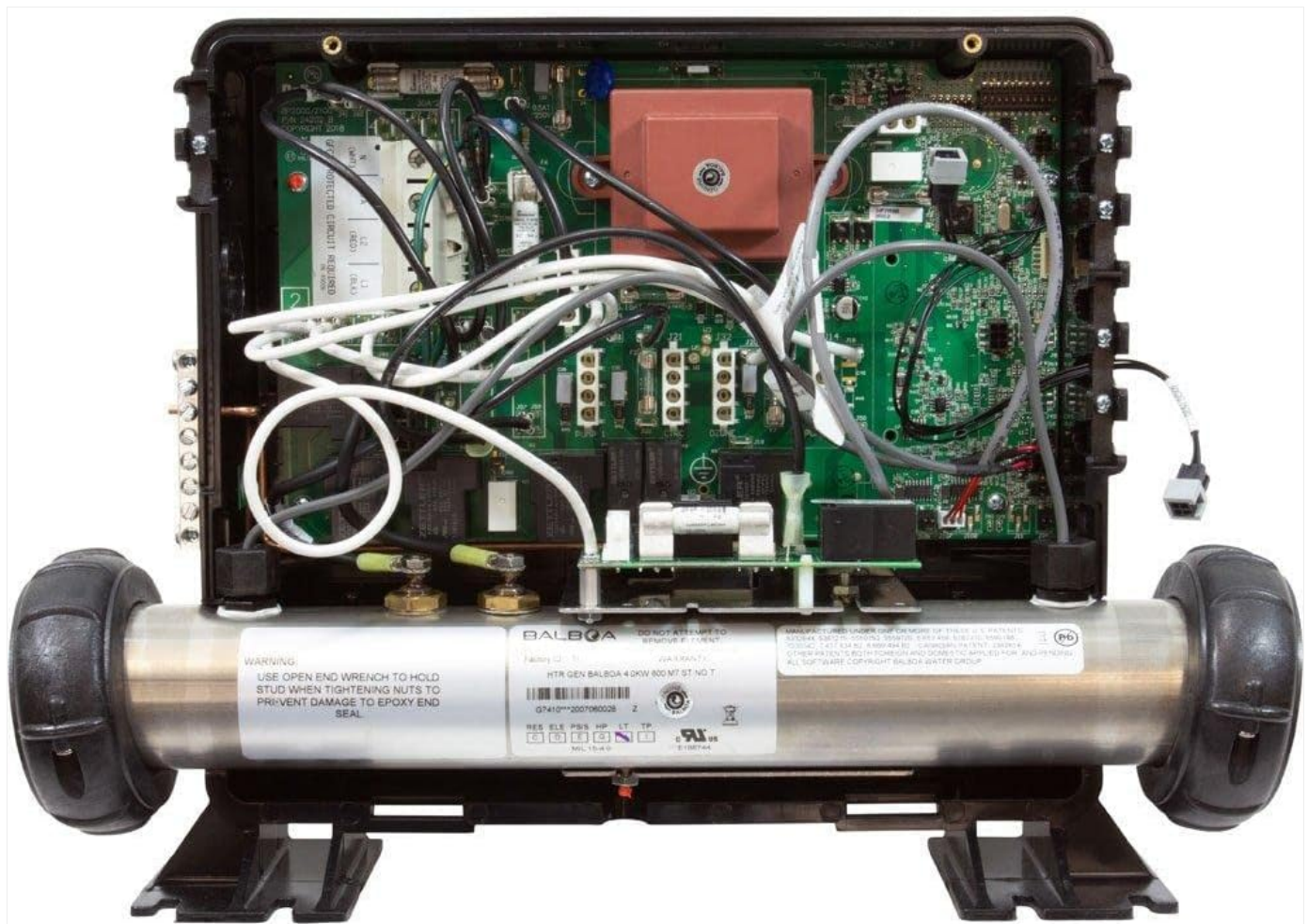
Image: Internal view of the Balboa BP7 Control System, showing wiring and components.
