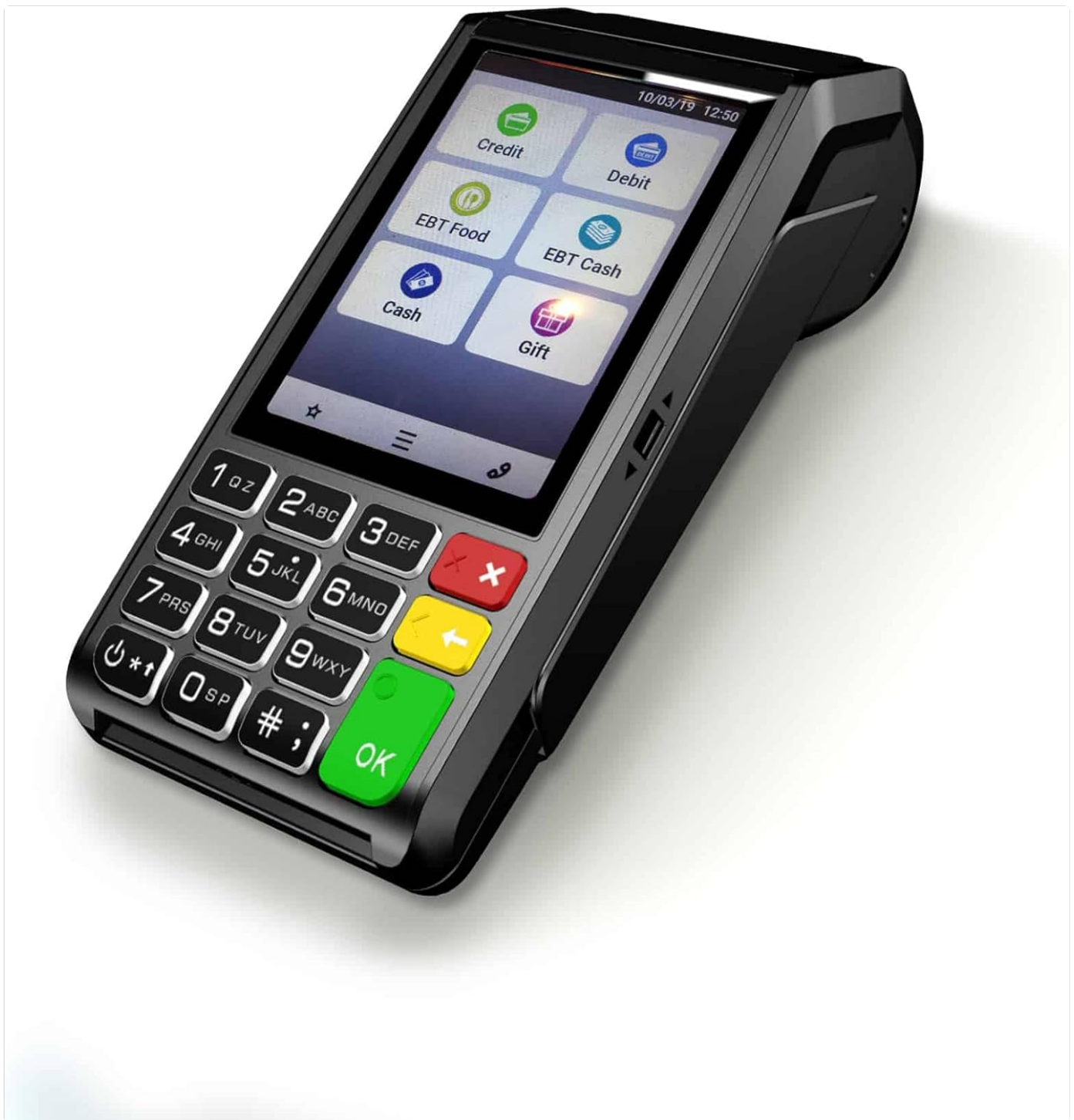
Figure 3.1: Dejavoo Z9 4G EMV CTLS Portable Credit Card Terminal. This image displays the black portable credit card terminal from an angled perspective, showing its color touchscreen interface with various payment options (Credit, Debit, EBT Food, EBT Cash, Cash, Gift) and a numeric keypad with function keys (red 'X' for cancel, yellow arrow for backspace, green 'OK' for confirm).
