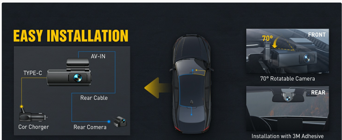
Image 3.1: Easy installation diagram for the EUKI X11 Dash Cam.
