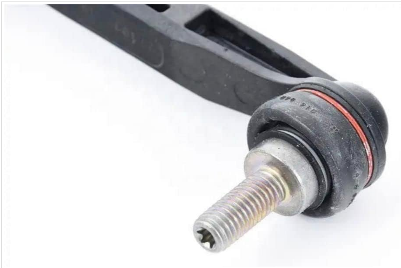
Image 3: Close-up view of the other end of the connecting rod, featuring a threaded bolt and a ball joint with a protective boot. This end also connects to a suspension component, allowing for rotational movement.
