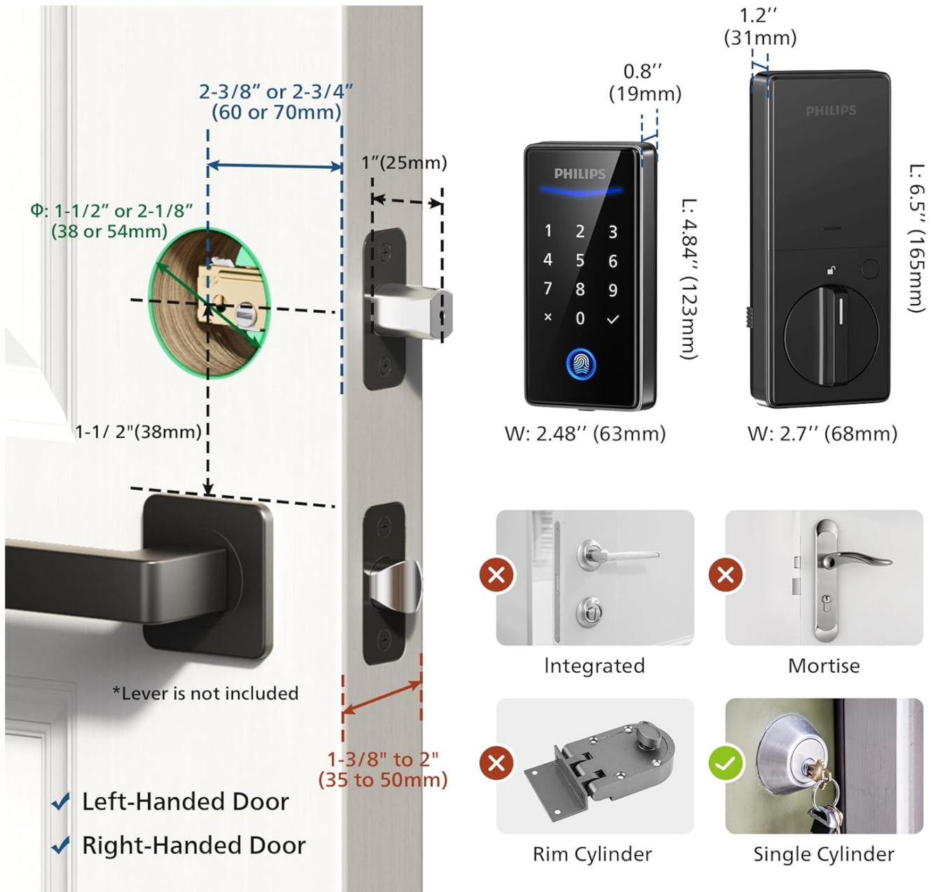
Figure 2: Door Dimension Requirements
