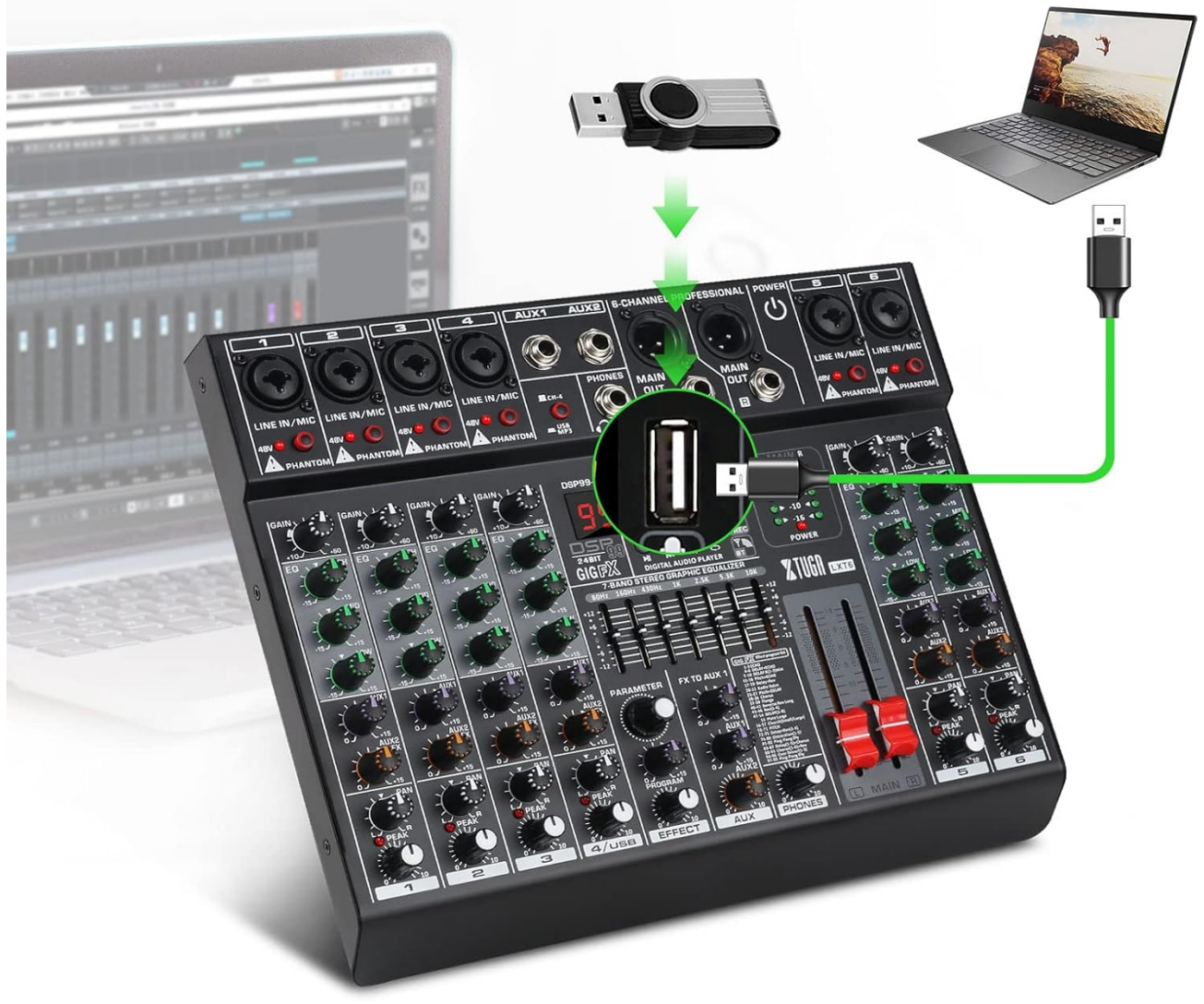
Image 3.2: Illustration of connecting the mixer to a laptop and a USB flash drive for digital audio functions.
